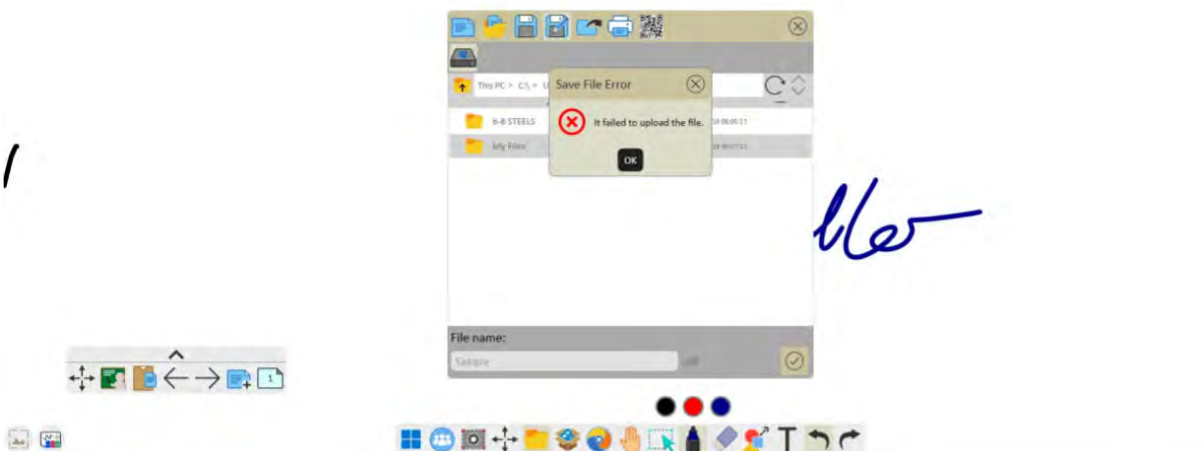
Save File Error message the user may encounter if they are not running myViewBoard Whiteboard as an administrator.
